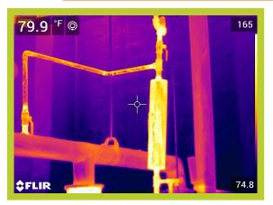
Operating Temperature, Ambient Temperature, Insulation selected 165\*F 67\*F Fiberglass
