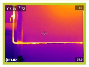
Operating Temperature, Ambient Temperature, Insulation selected 110\*F 67\*F Fiberglass
