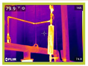
Operating Temperature, Ambient Temperature, Insulation selected 105\*F 67\*F Fiberglass
