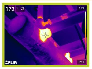
Operating Temperature, Ambient Temperature, Insulation selected 173\*F 67\*F Fiberglass
