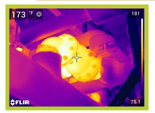
Operating Temperature, Ambient Temperature, Insulation selected 180\*F 67\*F Fiberglass Emittance of Surface
