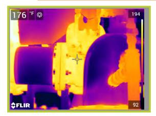
Operating Temperature, Ambient Temperature, Insulation selected 180\*F 71\*F Fiberglass Emittance of Surface0.95Expected Useful Life of Insulation System20 yrs.Operating hours per year8760Efficiency of fuel Conversion%85%
