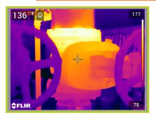
Operating Temperature, Ambient Temperature, Insulation selected 180\*F 71\*F Fiberglass
