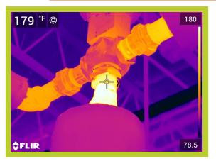
Operating Temperature, Ambient Temperature, Insulation selected 180\*F 70\*F Fiberglass Emittance of Surface Expected Useful Life of Insulation System Operating hours per year Efficiency of fuel Conversion% 0.95 20 yrs. 8760 85%
