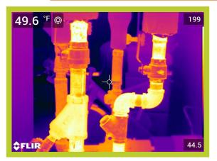
Operating Temperature, Ambient Temperature, Insulation selected 198\*F 70\*F Fiberglass Emittance of Surface0.95Expected Useful Life of Insulation System20 yrs.Operating hours per year8760Efficiency of fuel Conversion%85%
