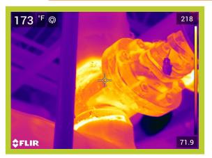
Operating Temperature, Ambient Temperature, Insulation selected 175\*F 70\*F Fiberglass Emittance of Surface0.95Expected Useful Life of Insulation System20 yrs.Operating hours per year8760Efficiency of fuel Conversion%85%
