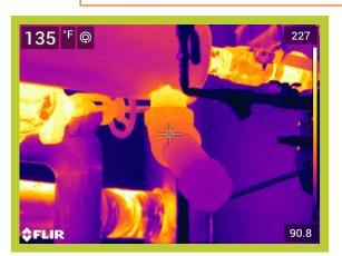
Operating Temperature, Ambient Temperature, Insulation selected 227\*F 70\*F Fiberglass
