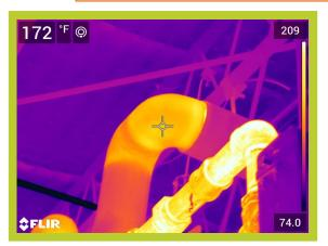
Operating Temperature, Ambient Temperature, Insulation selected 180\*F 70\*F Fiberglass
