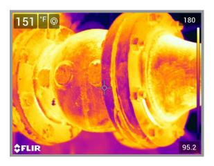
Operating Temperature, Ambient Temperature, Insulation selected 168\*F 77\*F Fiberglass Emittance of Surface
