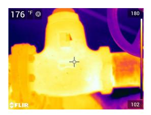
Operating Temperature, Ambient Temperature, Insulation selected 157\*F 77\*F Fiberglass Emittance of Surface
