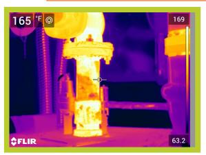
Operating Temperature, Ambient Temperature, Insulation selected 155\*F 62\*F Fiberglass
