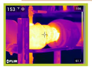
Operating Temperature, Ambient Temperature, Insulation selected 155\*F 62\*F Fiberglass Emittance of Surface
