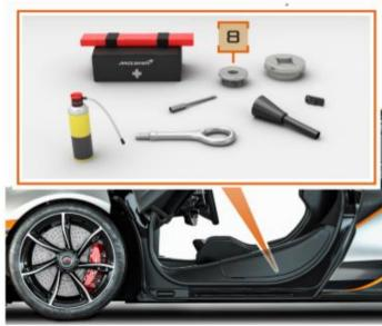
The locking ring removal tool (8) is located inside the accessories bag, behind the driver's seat.
