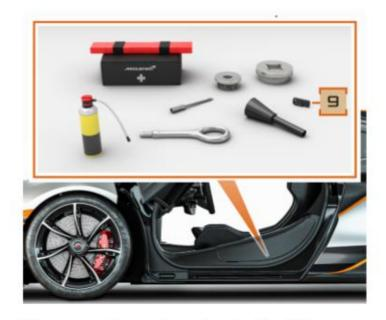
The manual door release key holder (9) is supplied with the vehicle.
