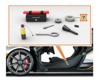
The center lock nut torque tool (7) is located inside the accessories bag, behind the driver's seat.
