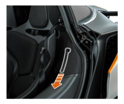
To release a door from inside, release the manual door release strap retainer and pull the strap.
