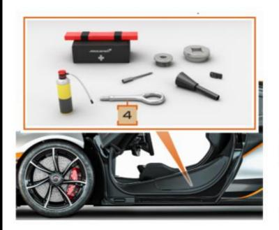
The towing eye (4) is located inside the first aid kit case behind the driver's seat.
