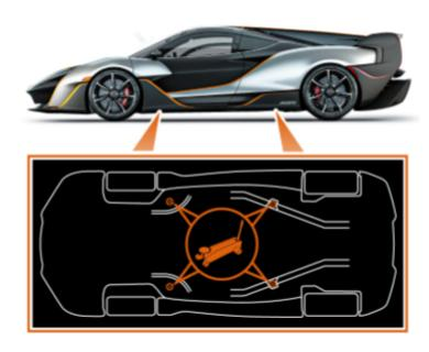
Refer to the illustration, and labels on the vehicle, for correct lifting locations.
