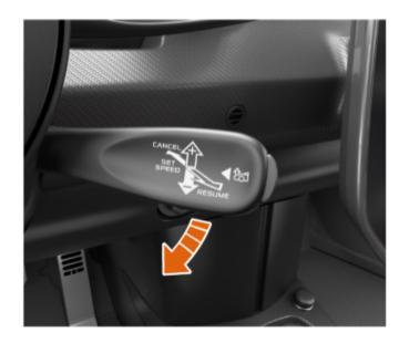
To lower the vehicle, activate the vehicle lift menu (see Vehicle lift operation, page 1.34) and then move the menu control stalk downwards.
