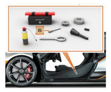
The front service cover release tool (6) is located inside the first aid kit case behind the driver's seat.
