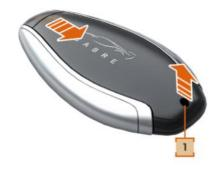
1. Remove the screw (1) and then slide the back cover away from the key fob.
