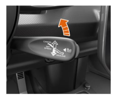
Before vehicle lift can be activated, the engine must be running. To raise the vehicle, activate the vehicle lift menu (see Vehicle lift operation, page 1.34) and then move the control stalk upwards.
