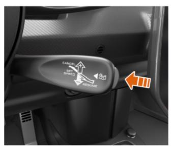
Access to vehicle lift is obtained by pressing the button on the control stalk on the right of the steering column, whenever the engine is running and the doors are closed.
