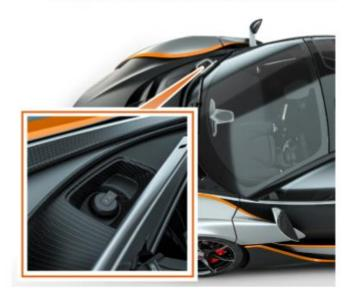
Refer to the instructions supplied with the battery charger. The charger connects to the accessory socket under the front service cover, see Front service covers, page 1.07.
