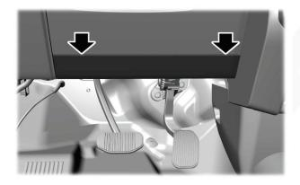
3. Carefully open the hinged access cover using a plastic type wedge or pry tool at the upper edge of the panel. If done correctly the panel will swing downward.
