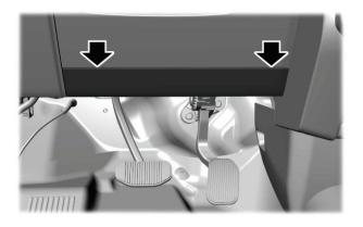
3. Carefully open the hinged access cover using a plastic type wedge or pry tool at the upper edge of the panel. If done correctly the panel will swing downward.
