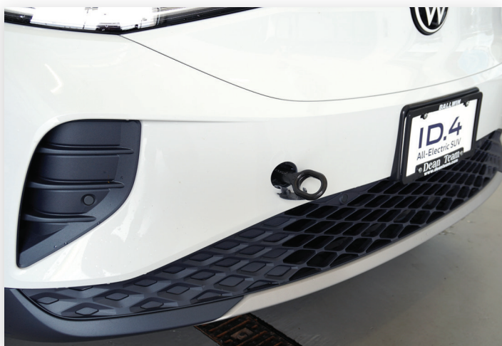
Tow eyelet is left-hand thread
