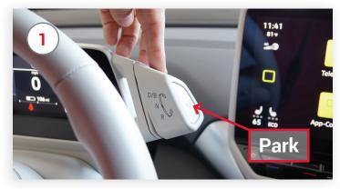
Enter the vehicle with key fob and depress foot brake. Shift vehicle to neutral by pulling the top of the shifter one click towards you.
