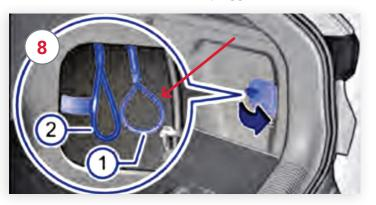
Pull Cord (1) in diagram to release charging cable.
