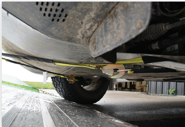
Nylon Bridle will lay flat on lower Front Bumper during loading
