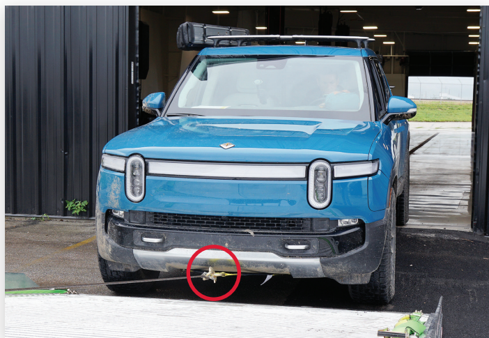
Nylon Bridle will lay flat on lower Front Bumper during loading
