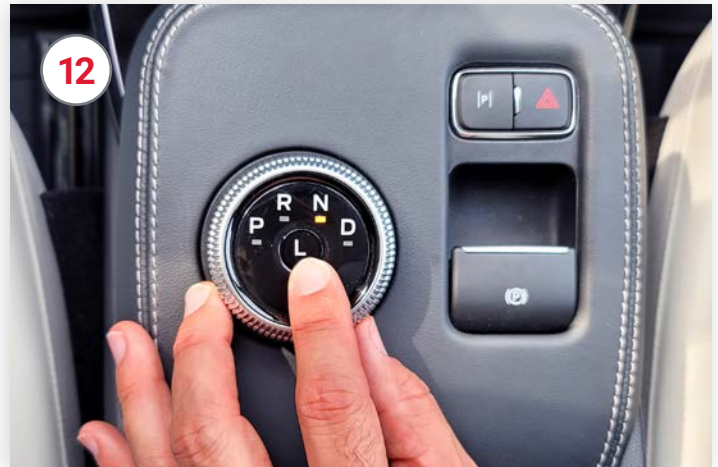
Press "L" in center of rotary shifter
