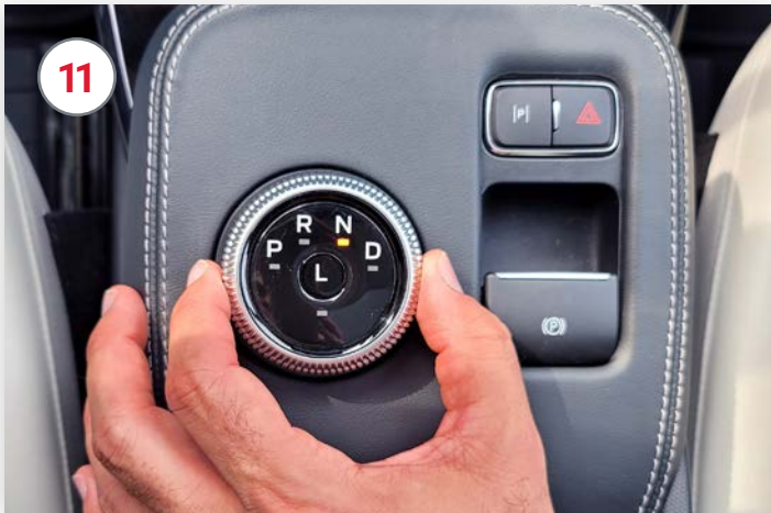
Shift vehicle to "N" Neutral with rotary shifter in center console
