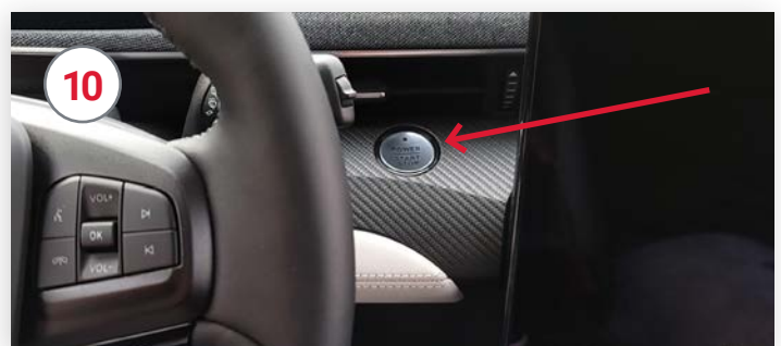
With Key Fob present press "Start" button to power up vehicle
