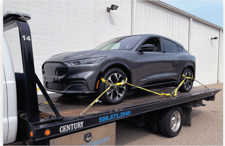
Retain and transport only using 8-point carrier kit
