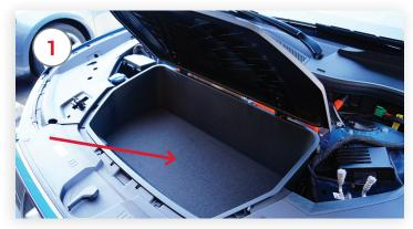
The Tool Kit can be found under the cargo floor of the front storage compartment, under "Hood"
