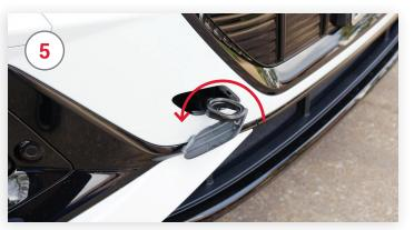
Tow Eyelet has Left Hand thread cut. Screw in Tow Eyelet to shoulder until it's seated in bumper beam
