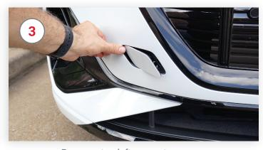
Press on top left corner to remove Front Tow Eyelet Cover
