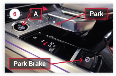
Enter vehicle with Key Fob present, depress foot brake, turn on vehicle with Start/Stop button (A)
