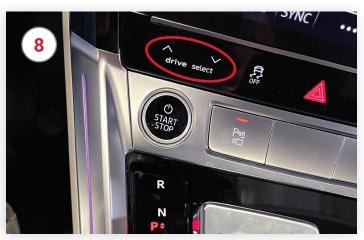
To raise vehicle prior to loading press "Drive Select" Up button
