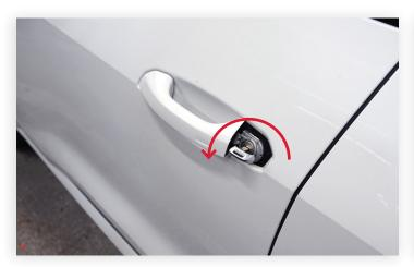
Insert Key Blade in Lock Cylinder Rotate Counter Clockwise
