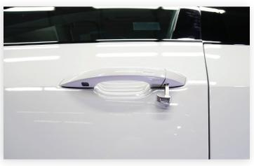
Insert Key Blade in slot in lock cylinder cover. *Gently* pull forward on key blade to remove cover.
