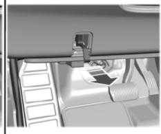
Using a tool or the key blade, carefully remove the access cover.
