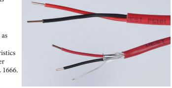
3. Type FPLP- FPLP power-limited fire alarm cable is listed by the NEC as being suitable for use in ducts, plenums and other space used for environmental air. All FPLP cable are listed as having adequate fire resistant and low-smokeproducing characteristics and must pass both UL test 1424 and UL Stiener tunnel test 910. (NFPA262)
