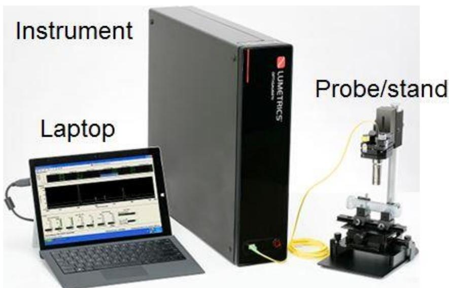
Figure 4. The Optigauge® II instrument along with a laptop computer for displaying and storing data on its left and a benchtop optical probe with stand on its right
