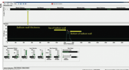
Fig. 1 – Optical signal obtained for the top wall of a medical balloon. The distance between the signal peaks is equal to the optical thickness of the wall.
