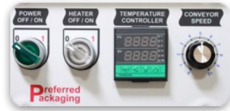
Tunnel Control Panel
