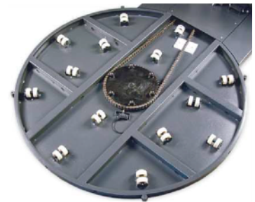
Heavy duty chain drive on turntable with 14 sets of double roller turntable supports. No maintenance or lubrication required.
