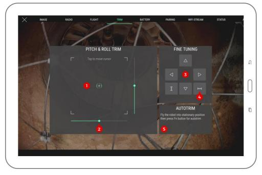
This panel allows the user to trim the drone should it be horizontally-drifting. Various controls are available to perform trimming.
