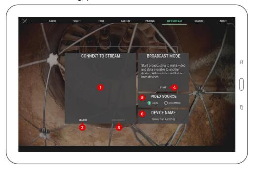
This panel controls everything related to data streaming between two devices through wifi. Wifi streaming allows using a secondary device as a simple viewer without needing to connect it to an actual remote controller; thus, two people can monitor a flight while using a single remote controller. Wifi streaming requires all devices to support Wi-Fi Direct.
