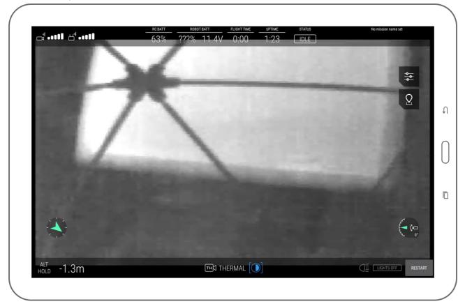
White displays the hottest and black the coldest area on the current frame. The range is always automatically scaled from the coldest to the hottest temperature measured on the current frame.
