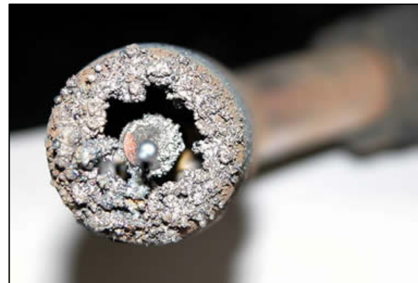
Spatter bridges against tip. Interfere with shielding gas and nozzle now electrically hot and disrupt shielding gas
