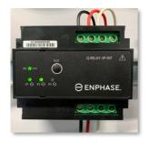
For each 25A solar circuit, L1 and L2 solar phases are connected into the 25A multi-phase Q-relay. The relay is programmed to 2-phases to satisfy interlocking requirements and perform loss of phase protection. The solar circuit neutral conductor(s) are also connected into the Neutral terminal at the Q-relay. A two pole 25A circuit breaker is required for each 25A PV solar circuit.
