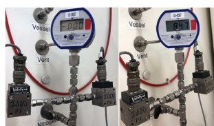
Figure 1: The FAI calibration tree with pressure gauge as the "calibrated source" for calibrating the pressure transducers. The left-hand-side shows the "zero"
