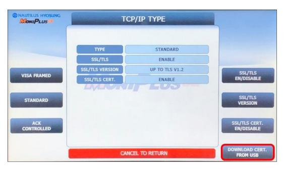
ATM Operator Menu > Customer Setup > Select Processor > TCP/IP Type
