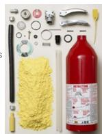
and then all parts including the chemical, cylinder, and any components are thoroughly inspected. If any parts require replacement, they are swapped out before the extinguisher is recharged and certified. Once the rebuild is finished, a verification of service collar shall be placed around the extinguisher's neck, and a label indicating the servicing company shall be affixed to the back.
