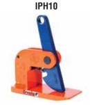
The IPH10 horizontal lifting clamps with spring loaded tension have a pretension feature that allows the user to attach the clamps to the material for horizontal lifting and transfer of nonsagging material. These clamps must be used in pairs or more
