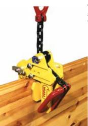
The NX is designed for lifting and revolving without marring of smooth or polished pieces such as stainless steel plates, aluminum, pre-lacquered plates, wood, laminated sheets, marble, concrete, glass, plastic or any other fragile surface.
