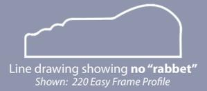
Frame adheres to the face of an existing mirror using industrial-grade double-sided tape.
