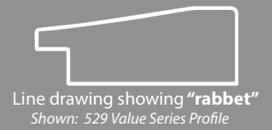
Manufactured with a special notch to allow a mirror to be glazed into the frame.
