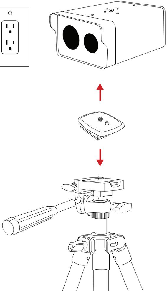
**MAKE SURE TRIPODS DO NOT BLOCK THE DIRECT PATH OF PERSON(S) TO BE IMAGED TO ENSURE THE EQUIPMENT WILL NOT BE MOVED OR KNOCKED DOWN. USING A DIVIDING BARRIER WILL HELP KEEP TRIPODS SEPARATE FROM THE PATH.**
