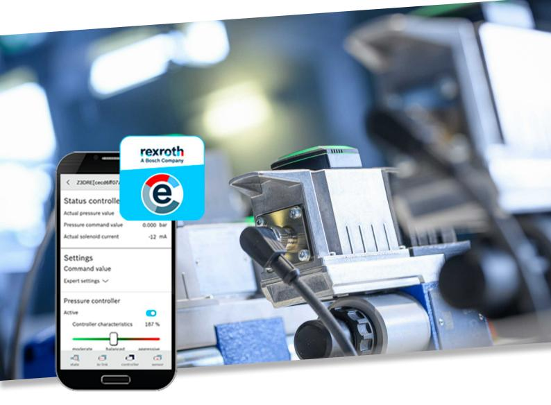
It has never been easier to configure hydraulic valves, set them to the optimum dynamics and read out error messages. Connect to the OBED digital control electronics of the Bosch Rexroth hydraulic valves with the easy2connect app independently of the control via Bluetooth. This speeds up commissioning, increases productivity and maximizes availability.
