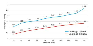
▲ 05 Rework vs. replacement: Leakage oil measurements on a prepared pump regulator (A4VSO) show significantly higher values than when replaced by the original component. Vibrations, increased wear and premature failure can be the result.
