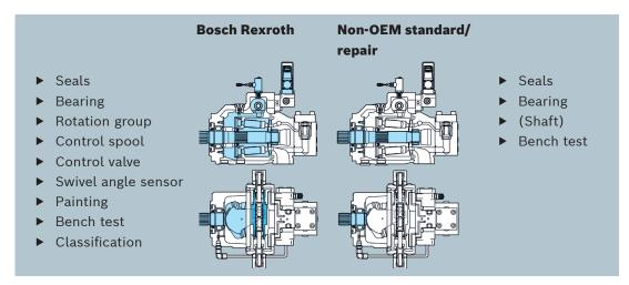
▲ 06 Repair comparison: In contrast to Bosch Rexroth, non-certified suppliers (right) only renew a few parts. Performance and service life of the pump are thus severely affected.
