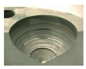
▲ 03 Surface comparison: In contrast to the original from Bosch Rexroth (left), the replica (right) shows large scores. The unfavorable flow conditions decrease efficiency. Leakage and cavitation are increased, especially under high pressure.
