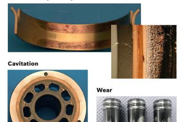
▲ 02 Fluid-related damage to various components of an axial piston pump.
