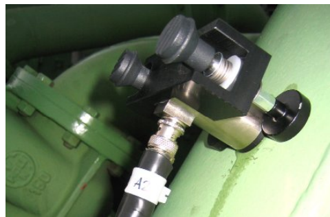
Acoustic sensor with magnetic holder
