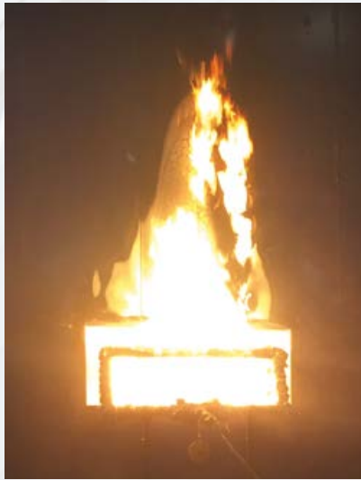
During the test a fire source simulates fire coming out of a window opening.
