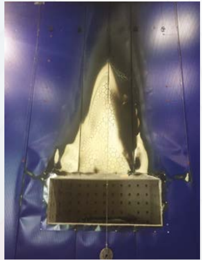
End of test showing the insulated panel system does not contribute to fire spread.
