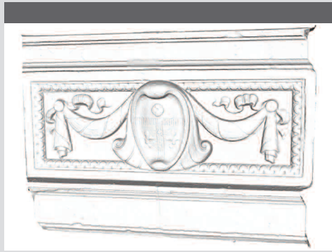
Figure 3: 3D model of spandrel panel developed with photogrammetry.
