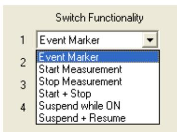
**Mark IV:** “Switch Functionality” is used to define the function of each pendant (available on Mark IV Portable profiler only). Up to four pendants can be used. Two plug into the Switch box while two plug into the EPU. In lieu of the pendants that plug into the switchbox, two buttons on the front of the switch box are provided. These are referred to as Switch 1 and 2. As can be seen in the diagram to the left, there are up to 6 assignable functions for each pendant/switch.
