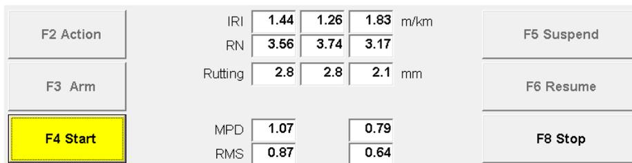
As shown above the operator still has the opportunity to initialize data collection manually by activating the **Start** button should the photo detector fail in detecting the trigger object.
