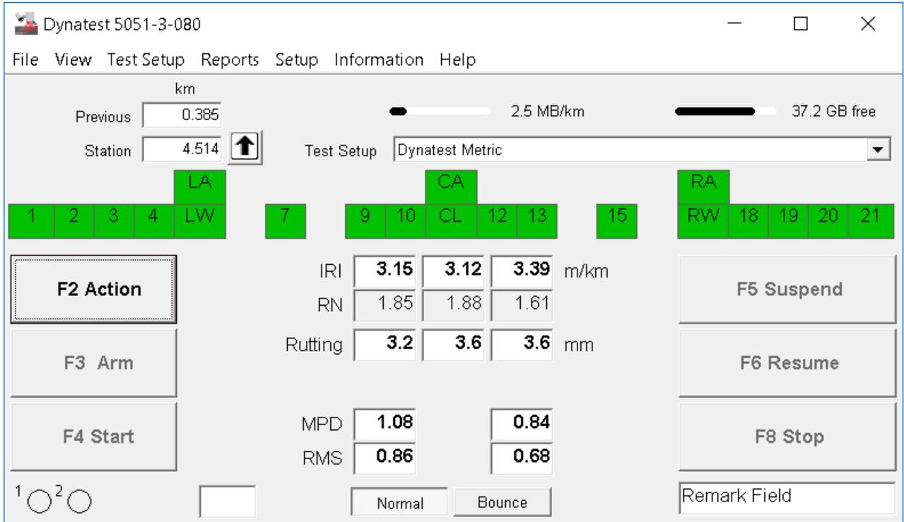
To make changes to the hardware setup, the user should click the **Setup** menu item along the top of the data collection screen. A drop down list of configurable items will appear as shown here:
