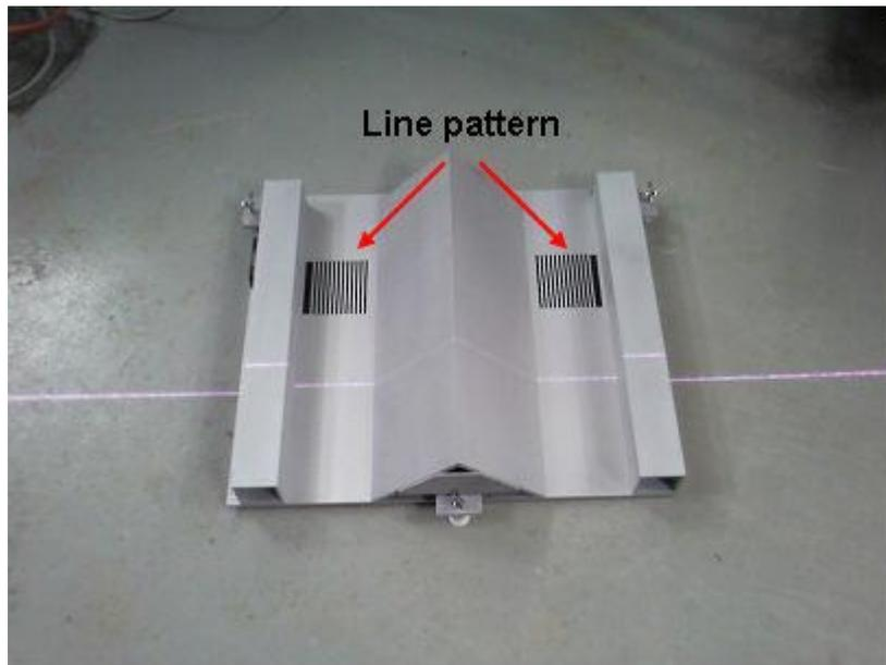
*Figure 37 Laser line position on the reference object for the Range Validation Test.*
