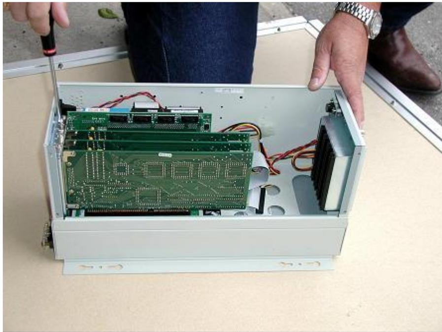
Press the PSB into the open slot. Secure the PSB with a screw.
