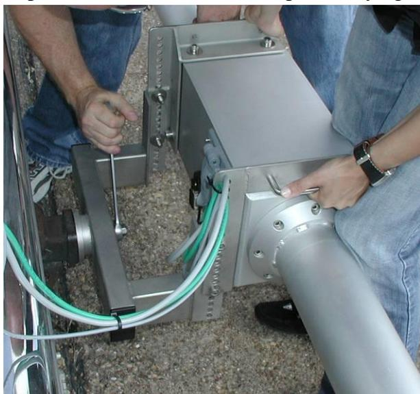
*Figure 18 - Securing the RSP to the hitch*
