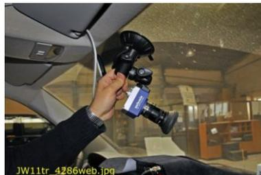
Press the rubber suction disk firmly against the window.
