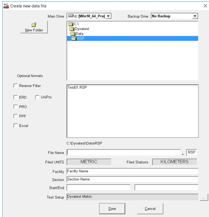
This dialog box allows the operator to navigate to an existing subfolder for file storage. It also allows the operator to create a **New Folder** and to select additional output formats and select a back-up drive (if applicable).
