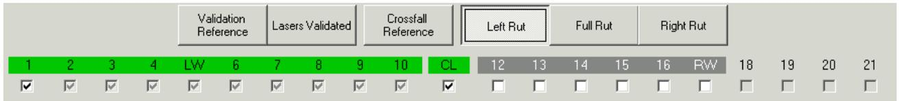
In the above figure Left Rut extends from channel 1 to 11 (from left side angled laser until centre laser). In all, channel 1 to 17 (from left side angled laser until right wheel (RW) laser) are available for the calculation of Left Rut.
