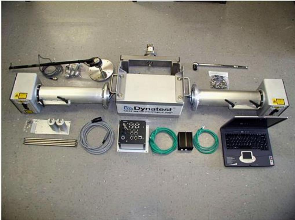
*Figure 12 - RSP Mark IV Components*
