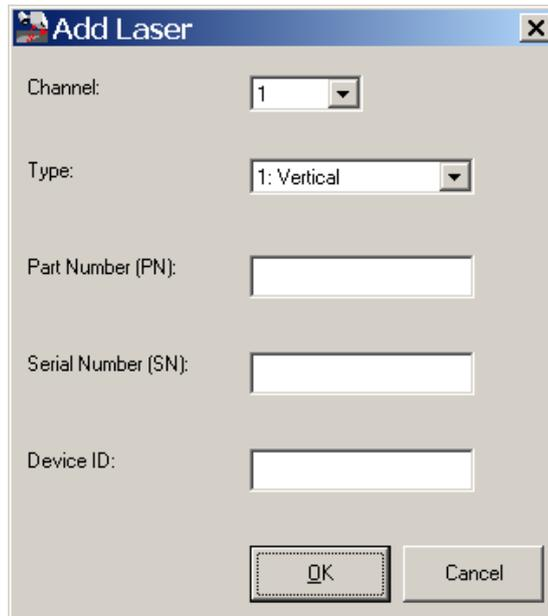
The Type, Part Number (P/N), Serial Number (S/N) and Device ID needed to install a new laser is provided by Dynatest upon delivery of the equipment or delivery of a replacement (or additional) laser. If you add a new laser to your equipment you will need to recalibrate the lasers, see “9 Calibration”.
