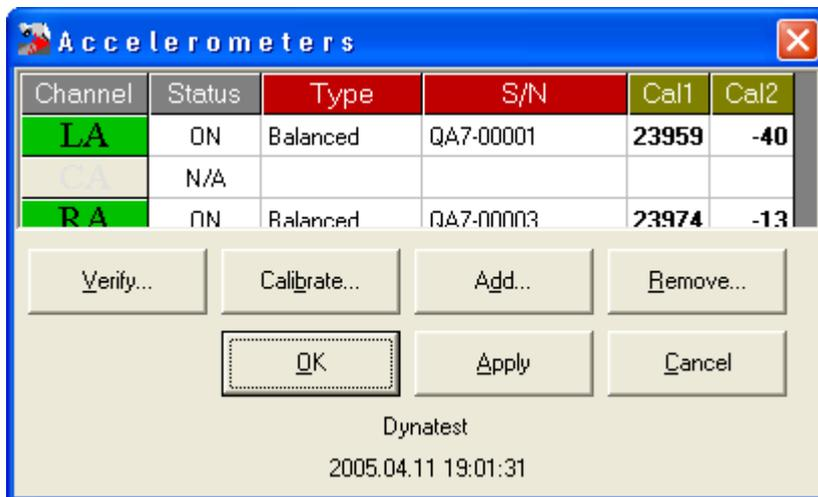
The bold numbers in the Cal 1 and Cal 2 fields in the windows above indicate that the net calibration values have not been stored. Click the “Apply” button to store the new values.
