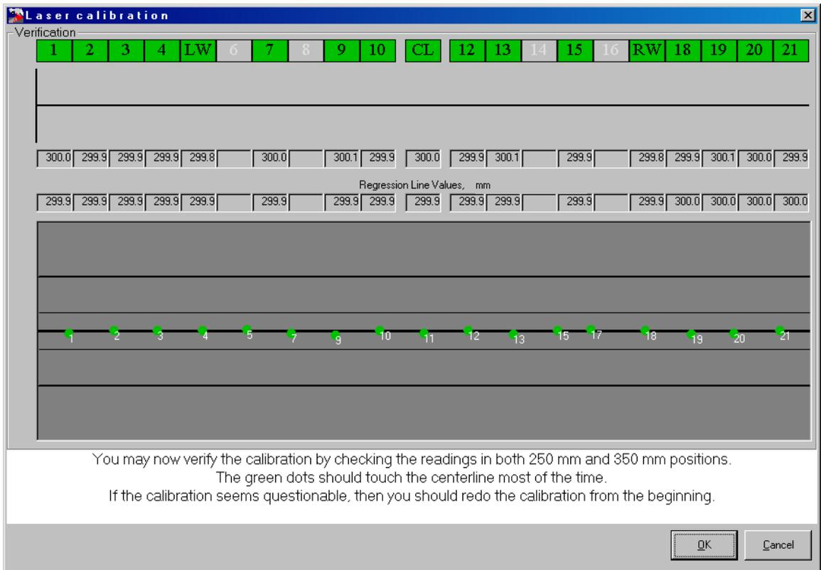
At this point the laser calibration is complete. Click **OK** to return to the main Laser setup window. In the Laser setup window you must click **OK** or **Apply** to the changes made to the Cal1/Cal2 and Pos1/Pos2 columns by the calibration procedure.
