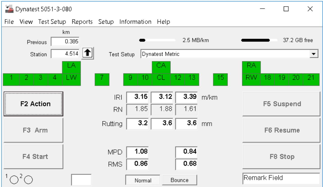
As mentioned earlier the Main window is the “mission control” for operation of the RspWin program. From this window the additional sub-windows can be toggled on and off by clicking the **View** menu item on the menu bar. Applets can be turned off from their individual menus.
