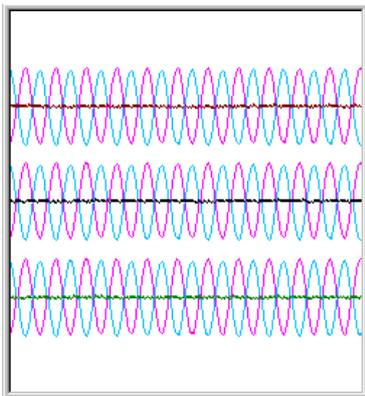
The cyan and magenta traces represent the lasers and accelerometers, which should be in opposite phases.
