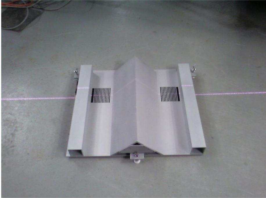
*Figure 39 Laser line position on the reference object for the Focus Validation.*
