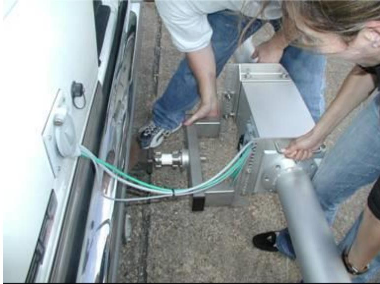
*Figure 26 - Installing the Transducer Bar*
