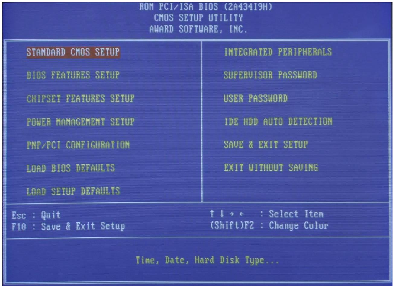
You will need to access STANDARD CMOS, BIOS FEATURES, CHIPSET FEATURES, PNP/PCI CONFIGURATION and INTEGRATED PERIPHERALS one by one and make changes as outlined in the following.
