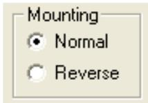
**Mark IV:** The Portable RSP Mark IV was intended for mounting at the back of the vehicle. If you occasionally mount the RSP at the front, then this option provides a convenient software swap of the Left and Right side data. There is no need to rearrange plugs or adjust other settings in RspWin. Just mount the RSP at the front and click the “Reverse” radio button. When you later re-mount at the back you must remember to reset this to “Normal”.
