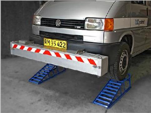
Raise the front of the vehicle so that the transducer beam is at least 500 mm (20 inches) off the ground. Make sure there are no disturbing vibrations. (Engine and fan turned off).
