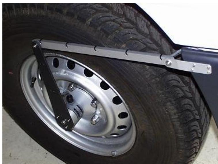
*Figure 11 - Typical Wheel Encoder Mounting*
