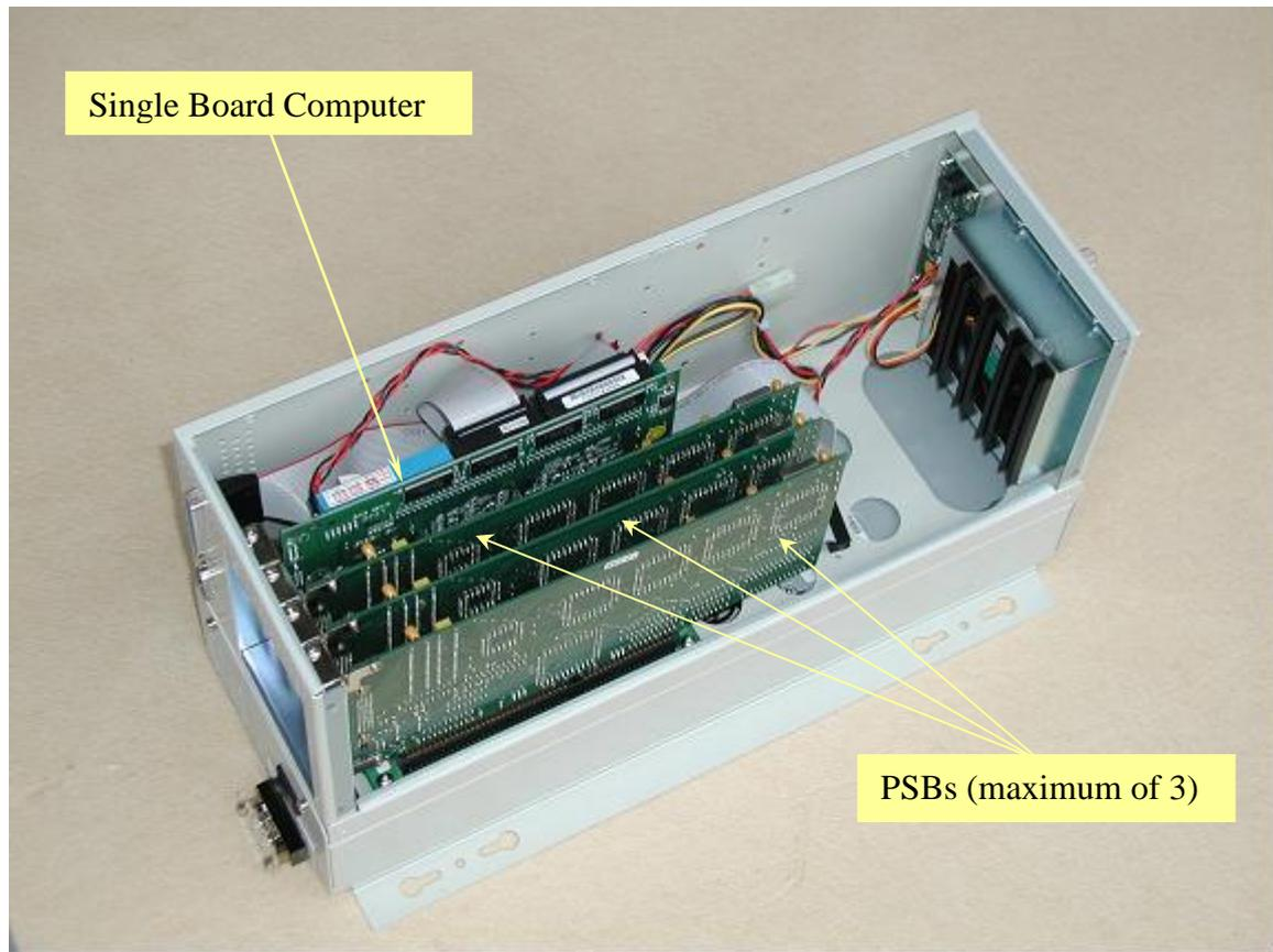
Once the PSB has been configured, it can be installed in one of the ISA slots. Simply remove the DPU cover, and then remove the screw and slot cover-plate from the back of the DPU.
