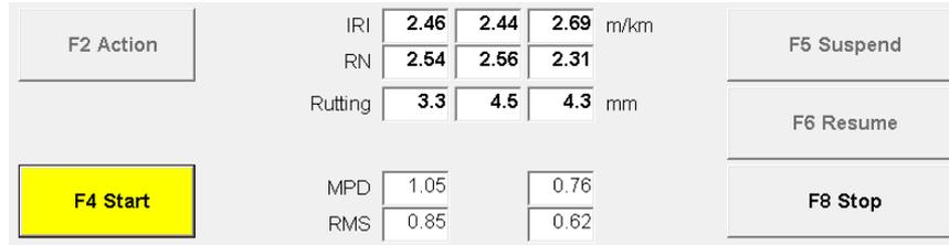
As shown above, all the command buttons except the **Start** and **Stop** buttons are greyed out. The focus is set to the **Start** button. Data collection will be initiated automatically, when the DMI reading reaches the "Start" value defined in the "Preparing ..." window. Since the **Start** button is not greyed out, the operator is still allowed to start the data collection manually, should he wish to do so.
