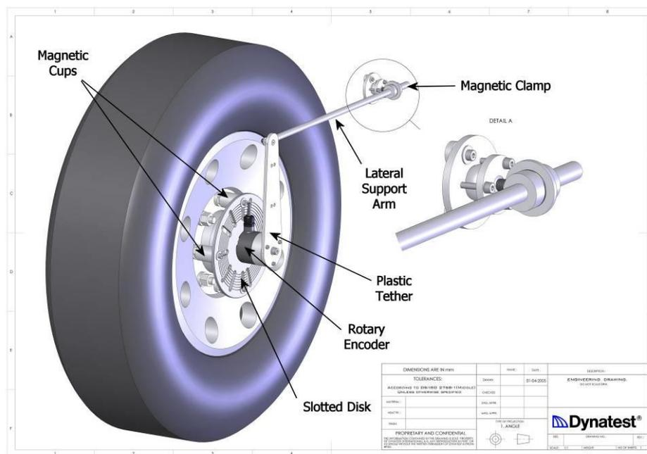
*Figure 31 - Wheel Encoder Schematic*
