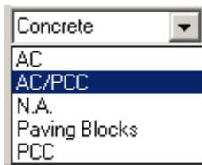
A combo box is a combination of a textbox and a drop-down list. The text portion of a drop-down list can only display items from the list, whereas a combo box allows the user to directly enter an input into the text portion as if it was a plain textbox as well.
