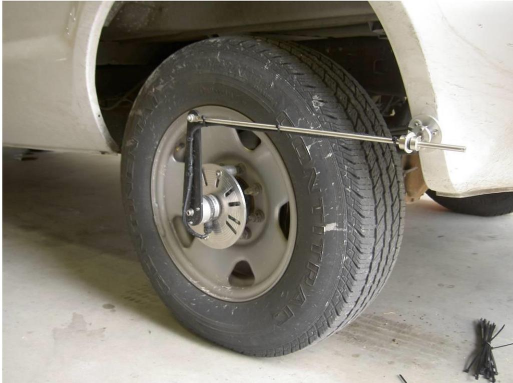
*Figure 23- Typical Portable Wheel Encoder Installation*
