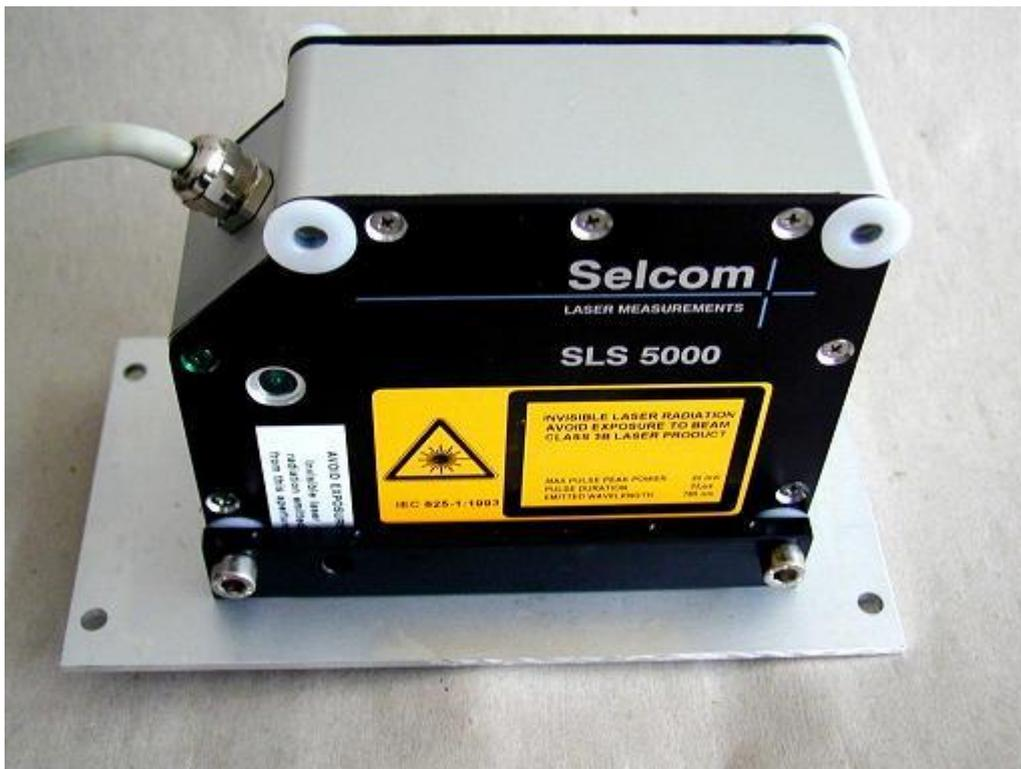
*Figure 4 - Selcom SLS 5000 laser module*
