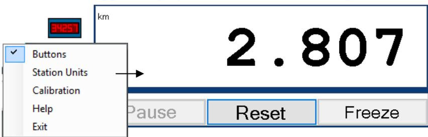
Uncheck “Buttons” to hide the Pause, Reset and Freeze
