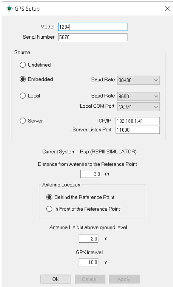
**Embedded** means that the GPS device is connected to DPU/EPU electronics. This is the recommended setup and achieves the best synchronization of DMI distance and GPS.
