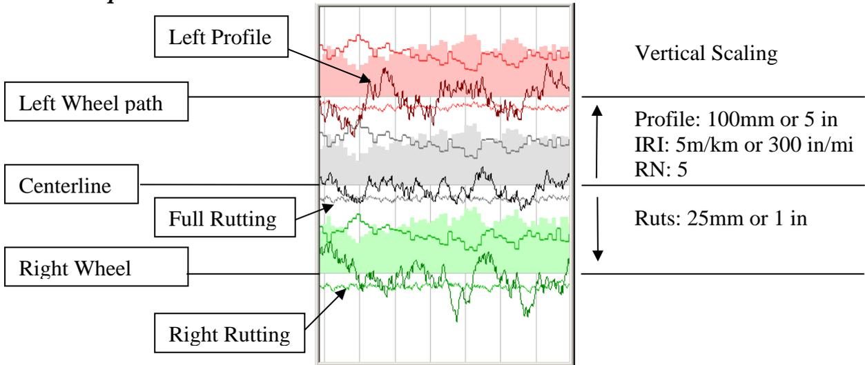
The Strip Chart rolls left across the window displaying Longitudinal Profile, IRI, Ride Number and Rutting. The filled column bars represent IRI values; the merely outlined column bars represent Ride Number. The vertical grey lines are spaced 0.1 km or 0.1 mile apart.
