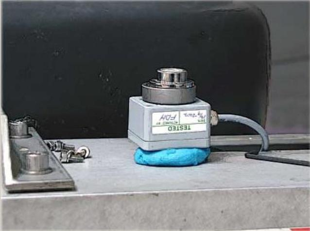
Place both accelerometers upside-down atop a ball of modelling clay. Place the level atop the accelerometers and push them down into the clay to flatten it. Adjust each accelerometer so that the bubble remains in the circle of the level.
