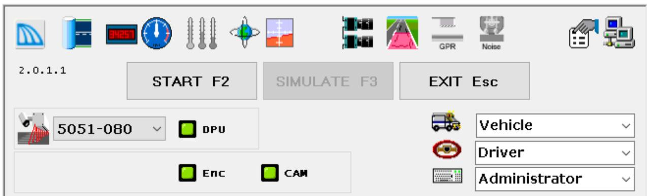
This sample shows that you will run tests with RSP 5051-080 and activate the following Applets: Network (roadway section database), DMI, Speedometer, GPS, IMS Inertial Motion Sensor (Gyro), Camera(s) and HDC (3D Crack Detection).
