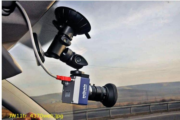
*Figure 40 ROW Camera Suction Disc Mount*
