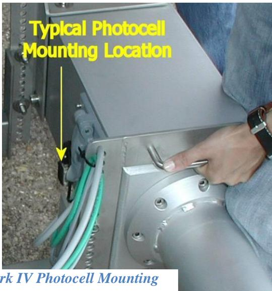
*Figure 21 - Mark IV Photocell Mounting Location*
