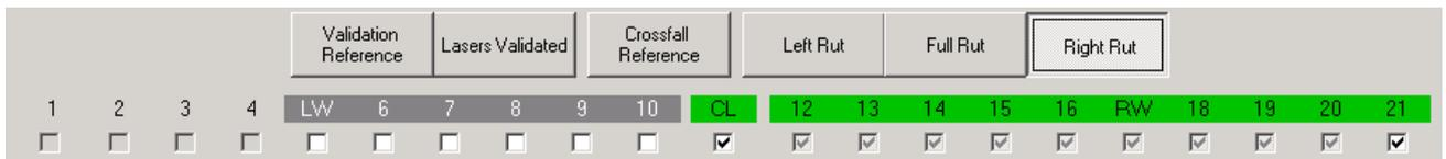
In the above figure Right Rut extends from channel 11 (centre) to 21 (rightmost angled laser). In all, channel 5 to 21 (from left wheel (LW) laser until right side angled laser) are available for the calculation of Right Rut.
