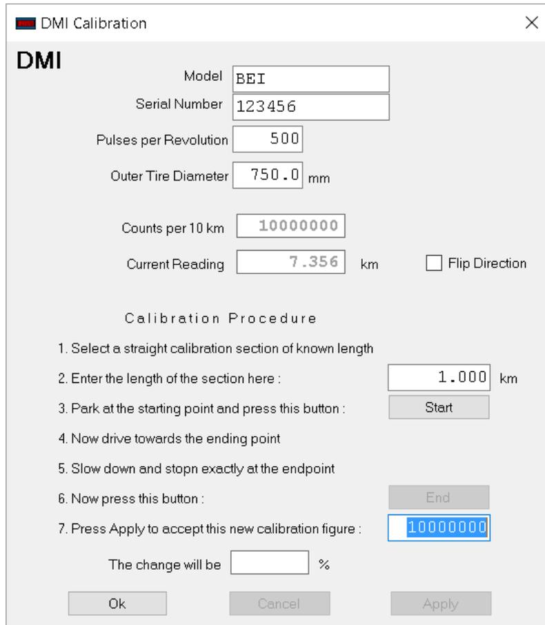
The calibration figure for the DMI is shown in the box labelled **Counts per 10 km**. This represents the expected total number of counts that would be accumulated over a distance of 10 km. The calibration figure is always displayed in units of **Counts per 10 km** regardless of the distance unit selected by the operator.
