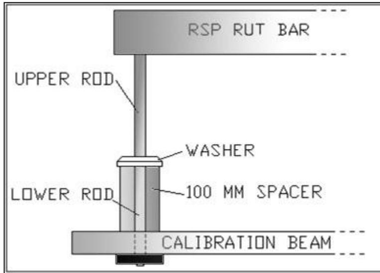
**Note:** The calibration should only be done where sunlight does not strike the beam - i.e. indoors if possible, otherwise in shade or cloudy weather.
