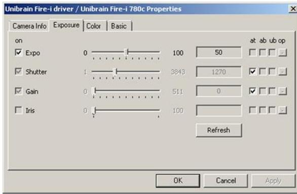
For “Shutter” as well as for “Gain”, check the “at” box.
