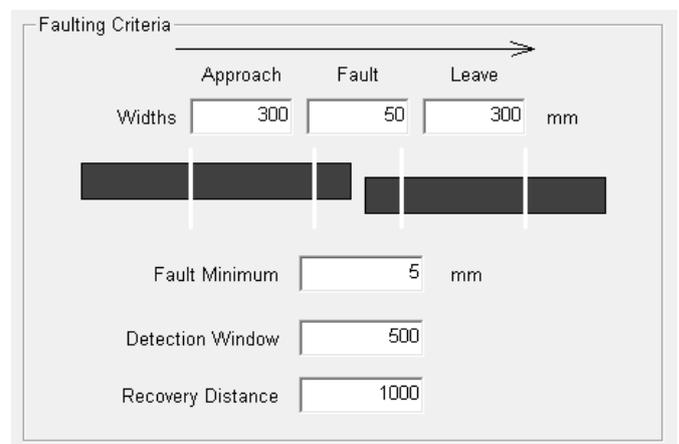
The detection algorithm has three phases: Approach (Lead), Fault (Drop zone) and Leave (Tail).
