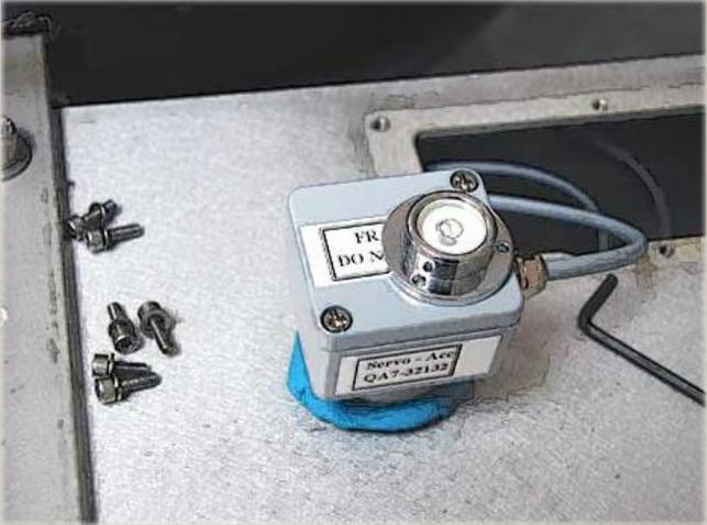
Turn the accelerometers over, place them atop the clay, and place the level atop the accelerometer. Adjust the accelerometer so that the bubble centers in the circle.
