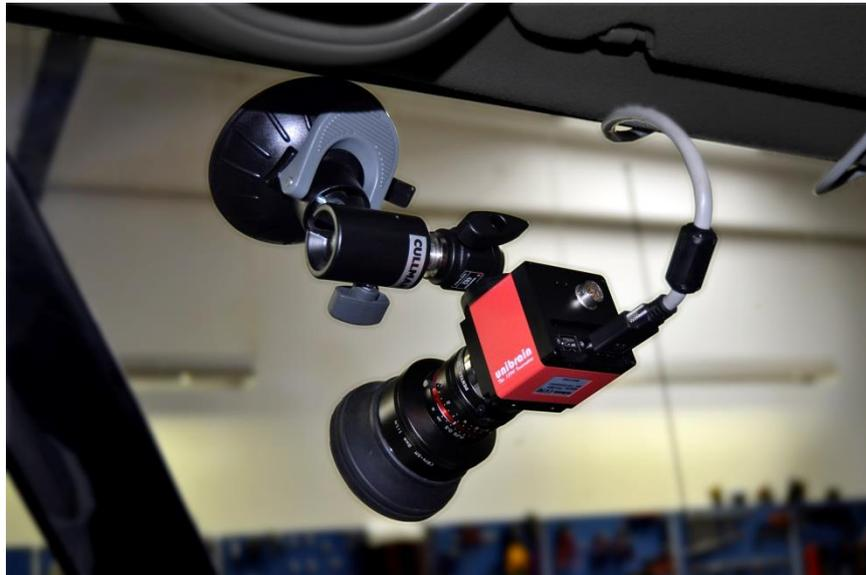
*Figure 33 - Digital Camera for Capturing Right of Way Images*
