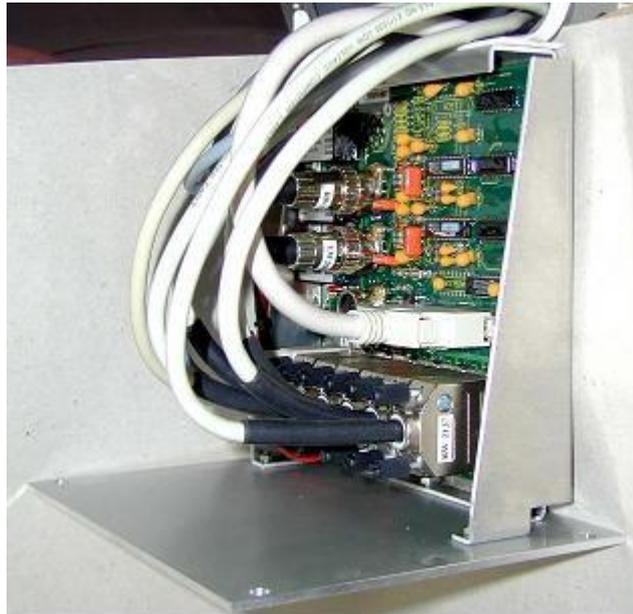
*Figure 8 - Primary Connection Module (PCM)*
