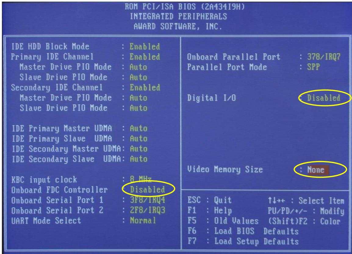
Finally choose SAVE & EXIT SETUP in the main setup window and confirm the decision. Switch off the system and then switch back on again.
