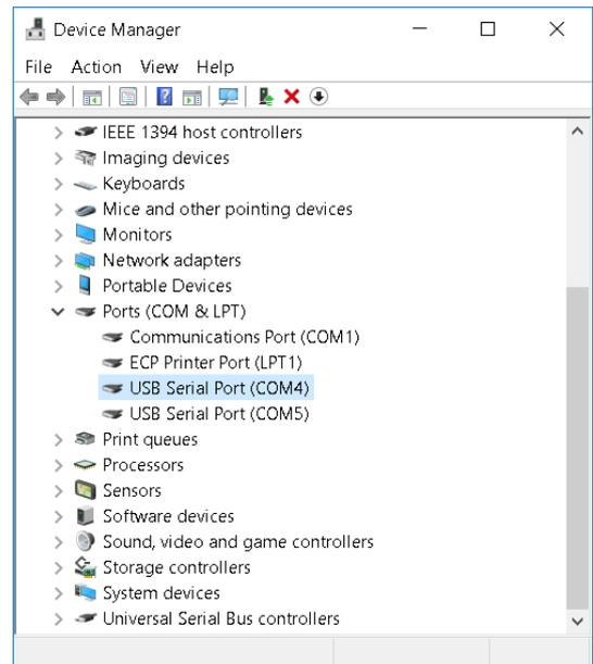
Right click each and go Properties – Port Settings – Advanced. Make sure that the Receive and Transmit bytes are set to 64 and that Latency Timer is 1 (lowest values).
