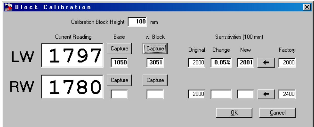
The factory-calibrated sensitivity can be entered by pressing the left-arrow.
