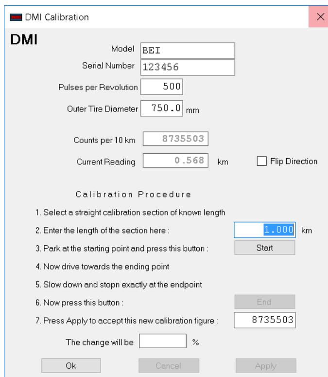
The first fields in the screen holds the encoder Model, Serial Number and advertised Pulses per Revolution.
