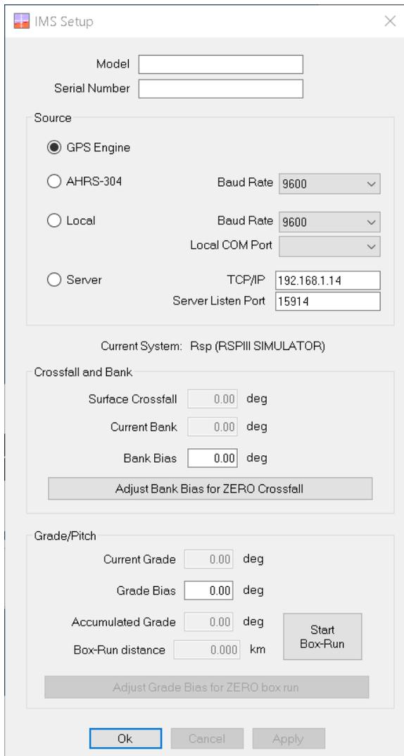
**GPS Engine** is for combined GPS/IMS systems like Applanix
