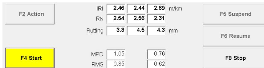
As shown above, all the command buttons, except the **Start** and **Stop** buttons, are greyed out. The focus is set to the **Start** button according to the "Start Mode" selected in the "Preparing ..." window. To initiate data collection you can either activate the **Start** button by pressing **F4** OR by pressing the **Enter** key.
