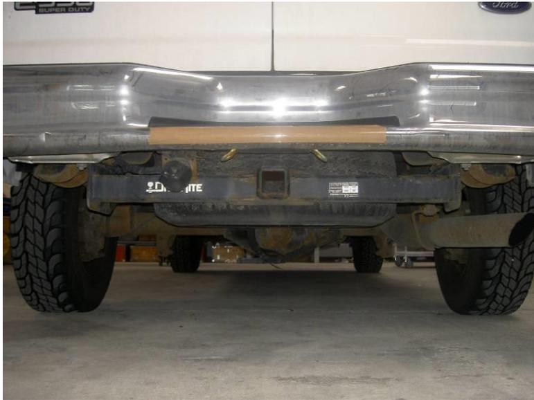
*Figure 24 - Receiver Style Hitch for RSP IV Mounting*
