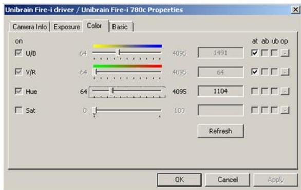
For “U/B” as well as for “V/R”, check the “at” box
