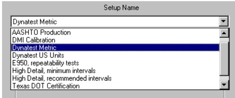
If you are happy with the selected setup click **OK** to exit the test setup window. If you would like to create a new setup or edit an existing one, you need to follow the guidelines below. Any changes you make will be stored in the active test setup displayed in the Setup Name field (if you press the **OK** or **Apply** command button).
