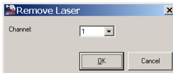
Be careful when completely removing a laser from the setup, since this procedure also removes the information needed to (re)connect the laser to your system. However there ARE situations when a user might want to remove a laser in order to reinstall it into a different channel. In that case, please remember to write down the Type, Part Number (P/N), Serial Number (S/N) and Device ID for the laser so that this data is available for the reinstallation.
