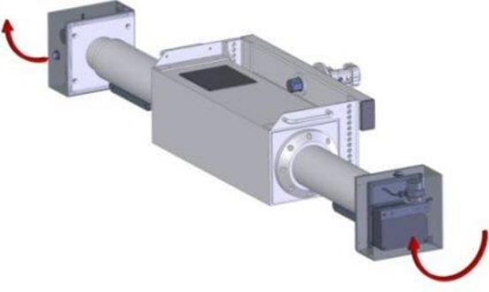
Rotate the laser enclosures to their upright (normal) position.
