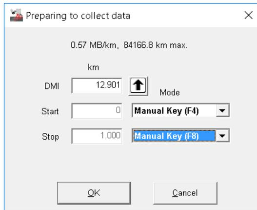
The "Start Mode" and "Stop Mode" fields are filled in according to what was specified in the test setup. However the user gets a last chance to make alterations to the Start/Stop modes and/or Start/Stop station fields (alterations made in the "Preparing ..." window will be remembered by the test setup).
