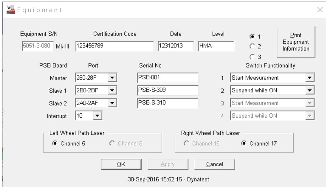
The first item to verify is the **Equipment Serial Number**. The serial number can be found on the nameplate located at the RSP transducer bar. If the serial number does not match your RSP, then you must restart RspWin. At the introductory screen, click on the correct equipment serial number, and then return to the above window. The equipment serial number should now be correct.
