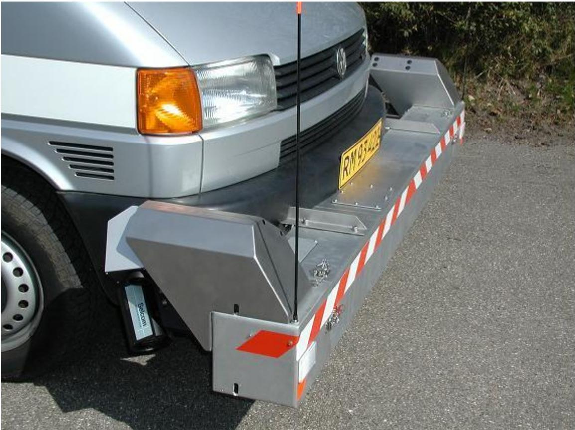
*Figure 3 - RSP Transducer Bar with Wing Extensions (L17.2)*
