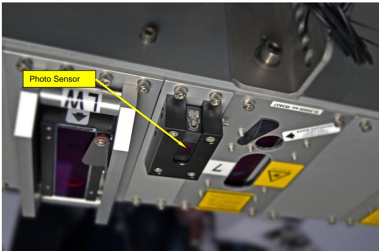
*Figure 7 - Photo Sensor Mounting Location*
