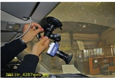
Apply suction with the lever and lock in position.
