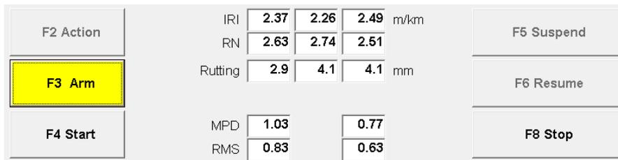
As shown above, the **Arm**, **Start** and **Stop** buttons are enabled. The **Arm** button is yellow and blinking, waiting to be activated. Since the **Arm** button has focus, you can activate it either by pressing **F3** OR by pressing the **Enter** key.
