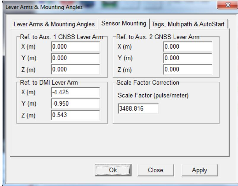
With Encoders generating 500 or 512 pulses/rev. the RSP DMI Calibration value shall be divided by 10,000 before entered into Applanix LV POSView.
