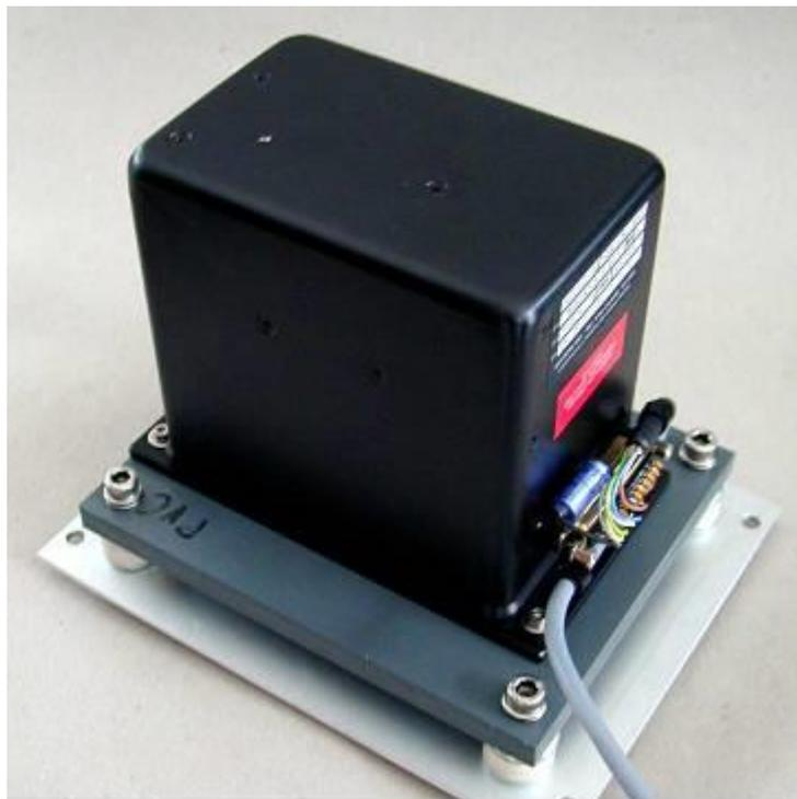
*Figure 6 - Watson AHRS E304 Inertial Measuring Sensor*
