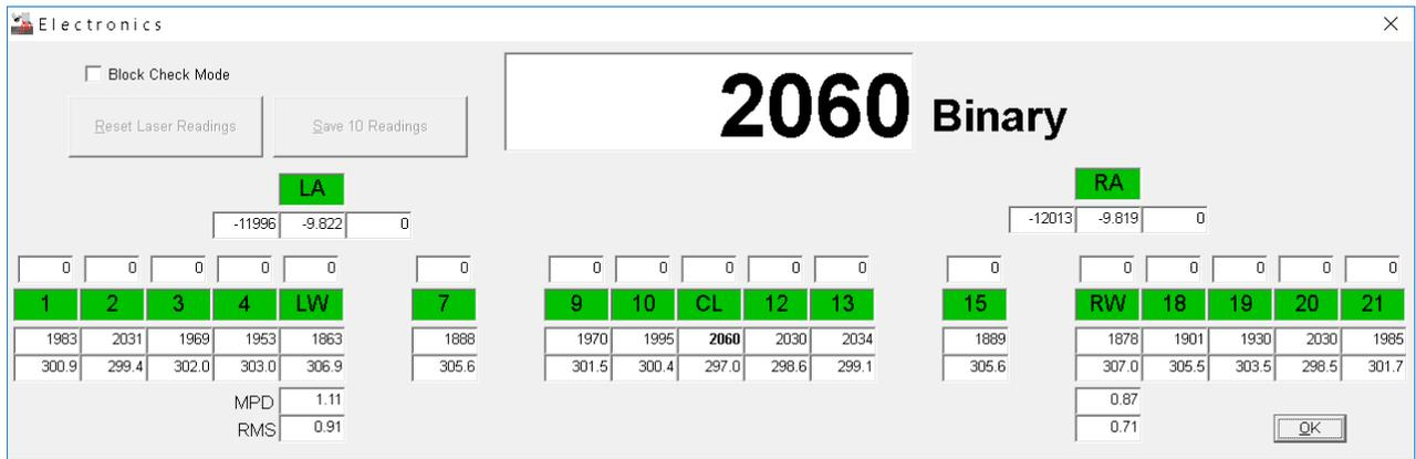
The fields below the accelerometer text boxes (LA, CA and RA) displays the raw accelerometer output readings (-12000), the accelerations as calculated by the program by making use of these readings (-9.81m/s<sup>2</sup>), and the percentage of bad/missing readings (0).
