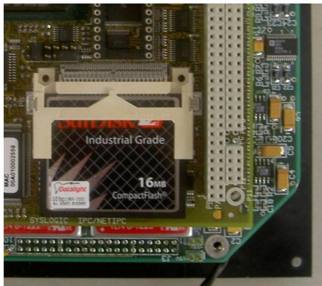
*Figure 16 - Flash disk inside the EPU*
