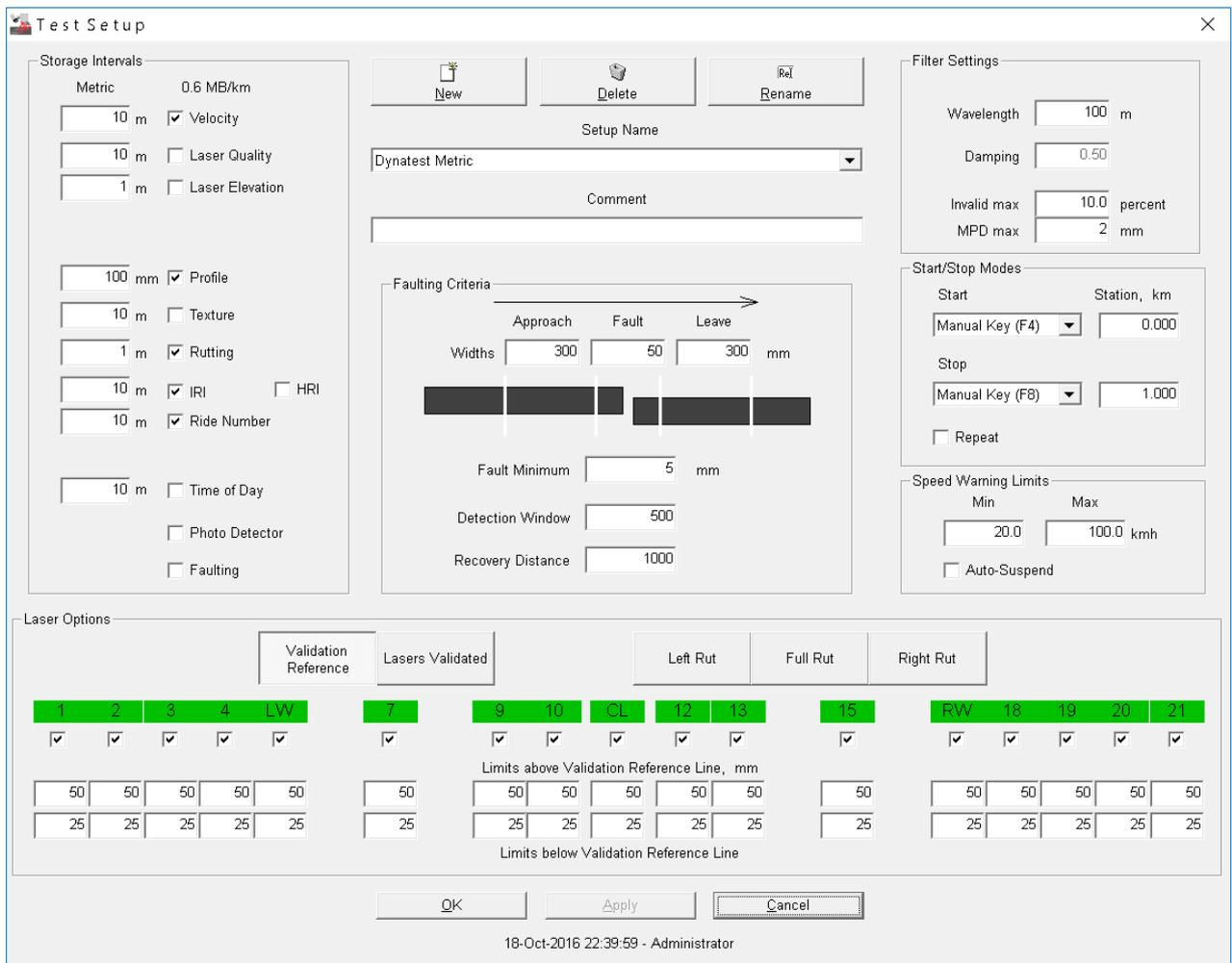
To select a different setup click the Setup Name combo box at the top of the test setup window.
