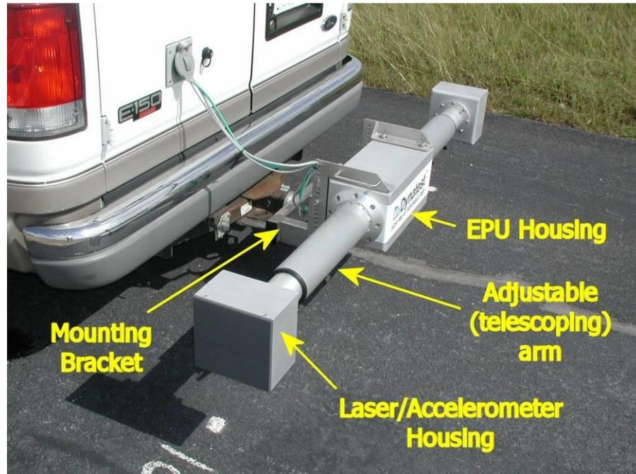
*Figure 17 - Mark IV Transducer Beam Components*
