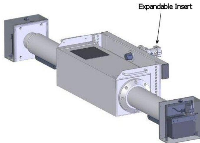
*Figure 25 - Transducer Beam with Insert*
