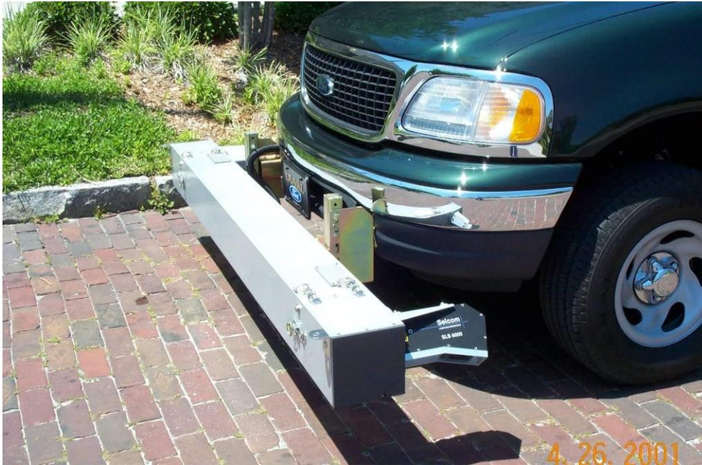
*Figure 10- RSP with Wing Extensions and Angled Lasers*
