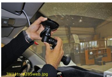
Pull back the plastic housing to protrude the rubber suction disk
