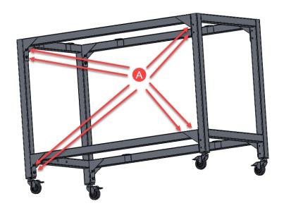
Insert bolts (16x) A tighten with a 9/16" wrench on all 8 corners.
