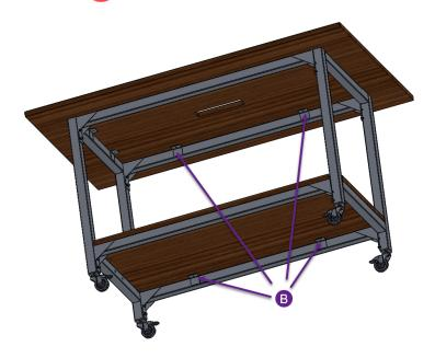
Place bottom shelf (4 screws) on first, then the top (8 screws), inserting (12x)
