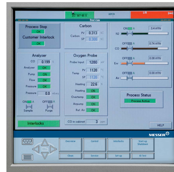
User-friendly customer interface for real-time monitoring and dynamic adjustment of furnace atmosphere
