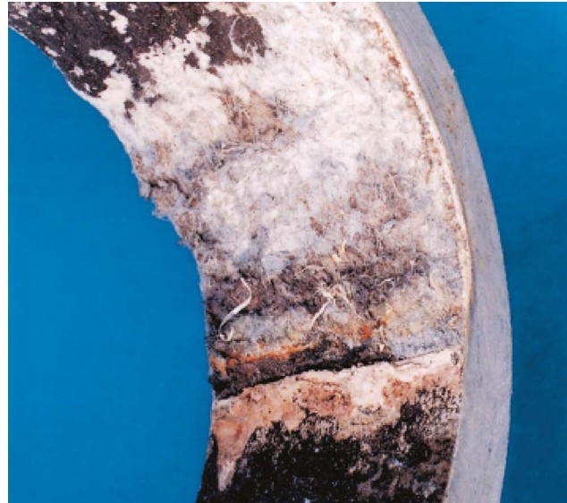
Costly: corrosion damage to a pressure pipe
