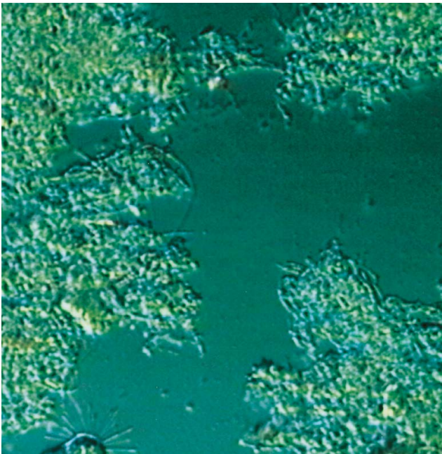
Well-developed sludge flocs after 14 days of oxygen treatment
