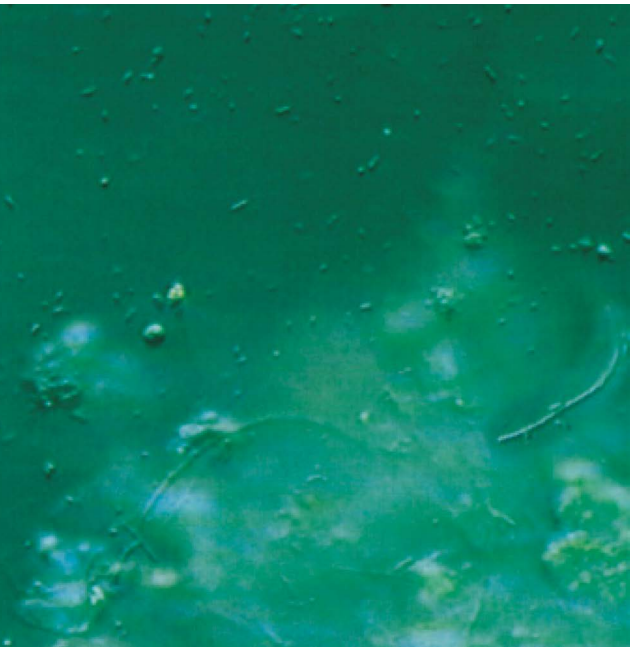
Weakly structured flocs caused by inadequate oxygen supply in the wastewater treatment plant of a brewery
