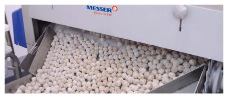
Pocino Foods quick freezes meatballs, pizza crumble and sliced and diced meat with the new Messer Wave Freezer from which features a patented rolling-wave action to keep products separate as they freeze.
