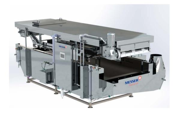
From chicken breasts to pizza toppings, strawberries to shrimp, the Messer nitrogen immersion freezer is the most reliable, accurate, and versatile compact freezer available for processing 1,000-15,000 lb/hr of individually quick frozen (IQF) food. Immersion freezing is the fastest way to freeze while locking important nutrients, moisture, and flavor into the food. The Messer immersion freezer can be adapted to specific processing needs to help increase the quality of frozen product.
