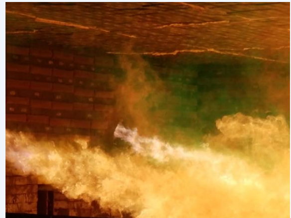
Working with Messer's combustion team, Hussey Copper increased production and refractory life by repositioning its OXIPYR burners.
