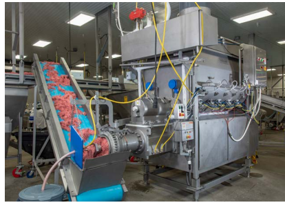
Chilled ground beef exits the mixer equipped with KRYOJECTOR injectors at right.
