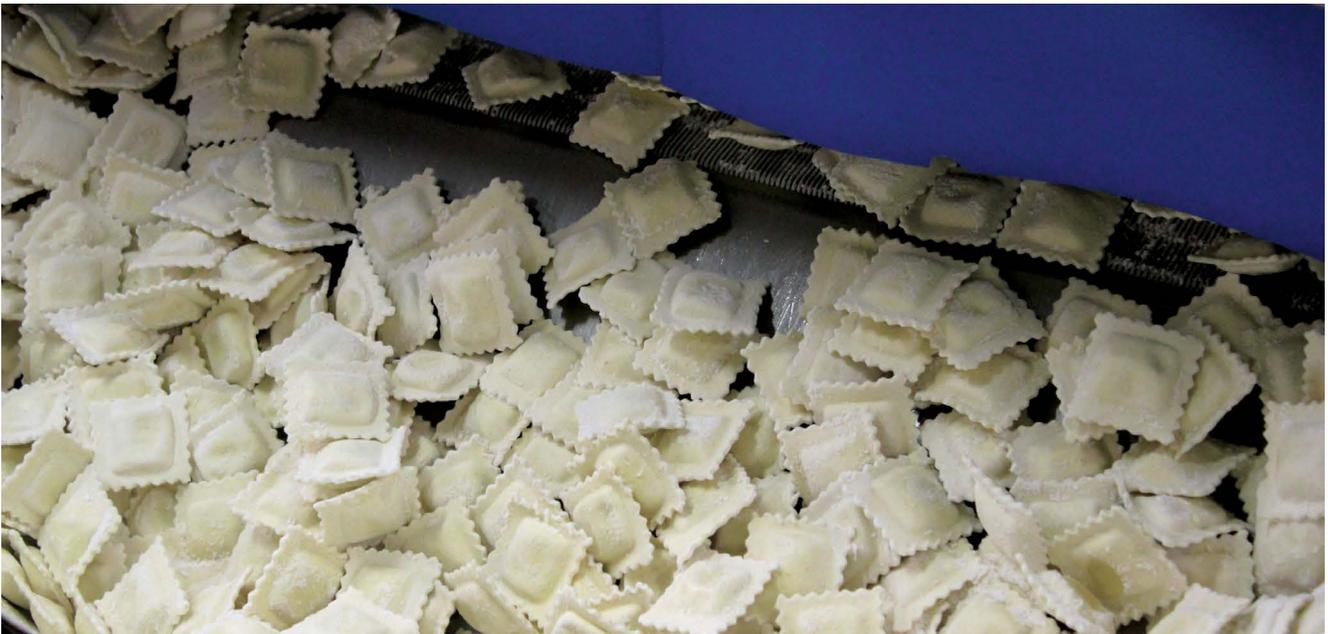
Pierino Frozen Foods, Inc. (Lincoln Park, MI) is one of the first prepared foods processors to harness new cryogenic 'rolling-wave' technology to individually quick freeze (IQF) gourmet pasta. The Messer Wave Freezer, patented by Messer (Bridge-water, NJ), uses a proprietary rolling-wave action to keep IQF products separate as they freeze.
