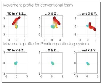
Spatial resolution improved from 5.6 mm to 4.9 mm and the average positional shift from one image to the next decreased by almost 40% from 0.17 to 0.105 mm.
