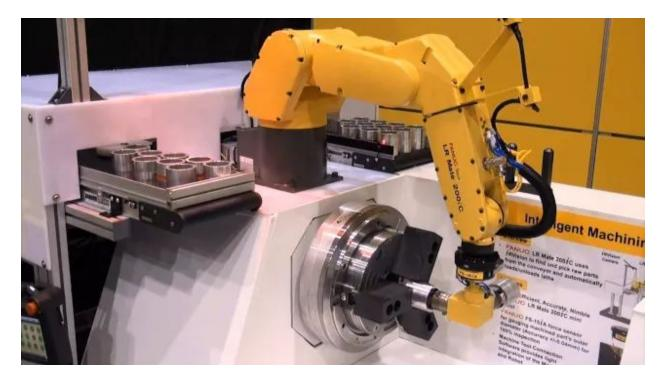
Video: Measuring a part's external diameter with a force-torque sensor.
