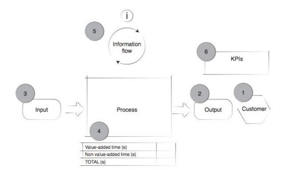
Robotic task map template. Numbers in circles indicate the order in which the information is to be filled.
