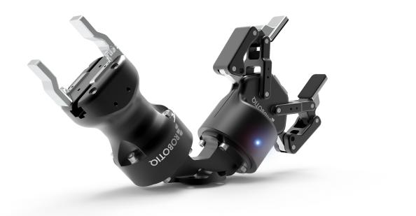
The most common reason why people will use a dual-gripper configuration is to improve cycle time. This is possible because a dual gripper lets you pick up multiple objects at once. When choosing the gripper for your application, you must consider:
