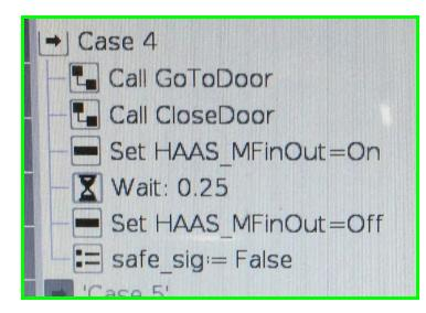
Here, the "Call" sequence means the user has called the subprograms "GoToDoor" and "CloseDoor".
