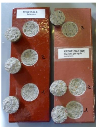
Fig. 2 Samples after adhesion testing.
