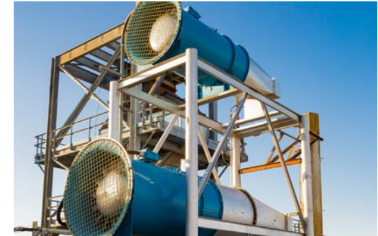
Pilot testing rig that simulates hurricane force winds and rain, and exceeds API 537 pilot testing requirements
