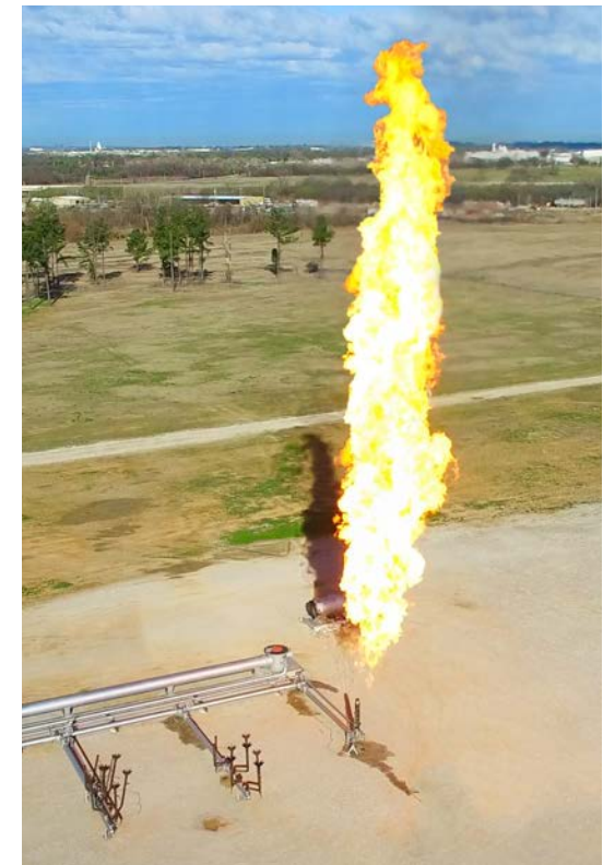
Pilot testing rig that simulates hurricane force winds and rain, and exceeds API 537 pilot testing requirements
