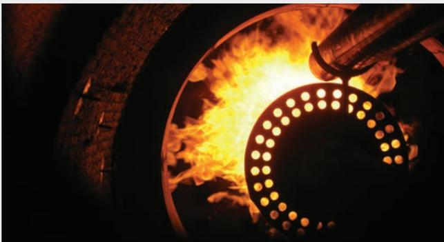
*ZEECO® thermal oxidizers reliably and safely destroy BTEX and amine acid gas streams with 99.999% DRE*
